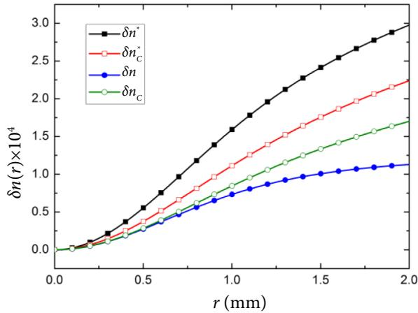
Fig. 4. Radial distribution of induced birefringence calculated using the simplified formula (hollow) and the full formula (solid) with standard (circle) elastooptic coefficients and an alternative set (square).
