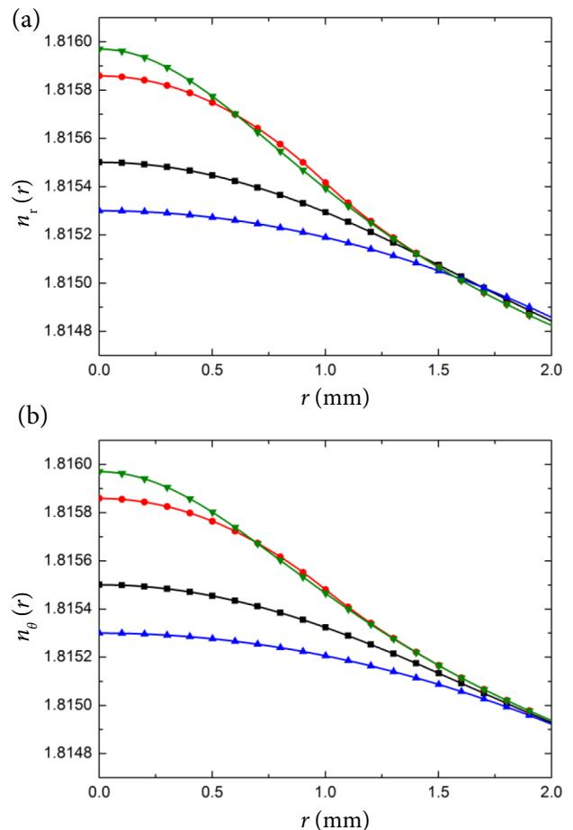
Fig. 2. Radial distribution of the radial (a) and the tangential (b) refractive index for uniform (up-pointing triangle, blue online), parabolic (square), top-hat (circle, red online) and Gaussian (down-pointing triangle, green online) thermal loading with the same total power.
