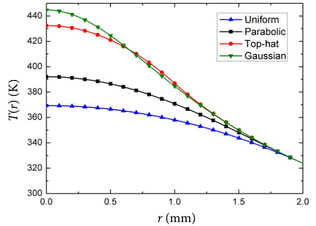
Fig. 1. Radial temperature distribution for uniform (up-pointing triangle, blue online), parabolic (square), top-hat (circle, red online) and Gaussian (down-pointing triangle, green online) thermal loading with the same total power.
