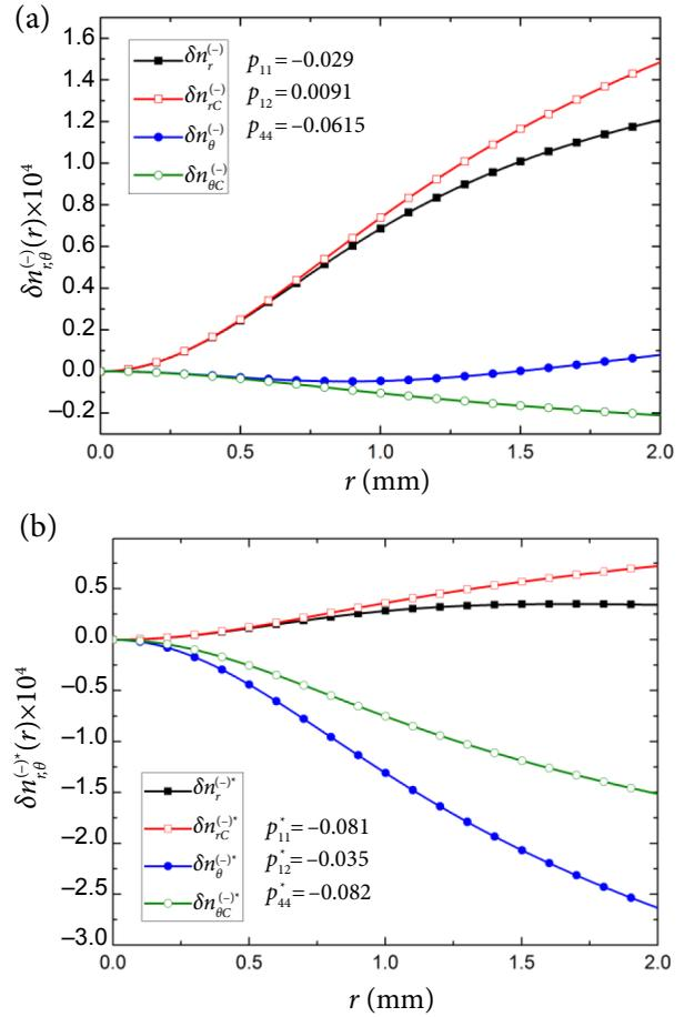
Fig. 3. Radial distribution of the radial (square) and the tangential (circle) refractive index difference due to the photoelastic effect calculated from the simplified formula (hollow) and the full formula (solid) using (a) standard elasto-optic coefficients and (b) alternative ones.
