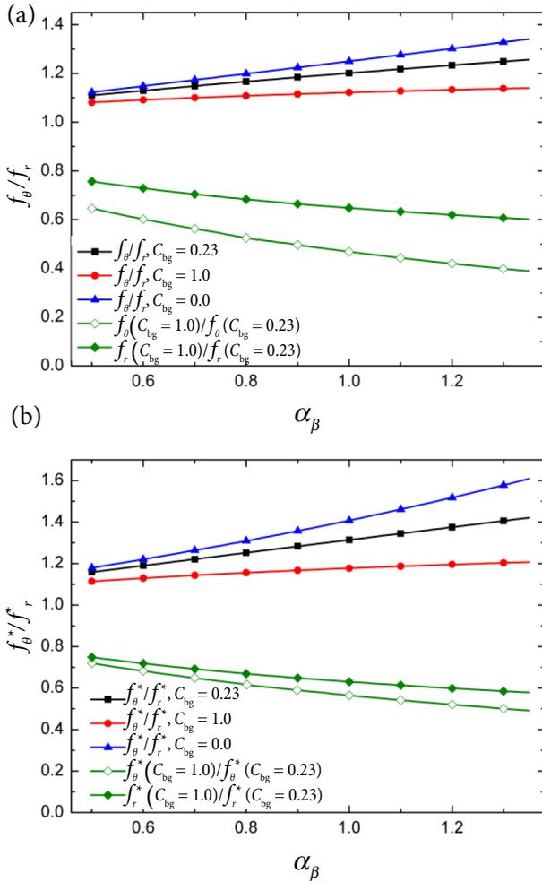
Fig. 6. Ratios of radial and tangential focal lengths for various approximations depending on the ratio of the thermal expansion coefficient to the thermo-optic coefficient at zero stress for (a) a set of standard elasto-optic coefficients and (b) an alternative one.
