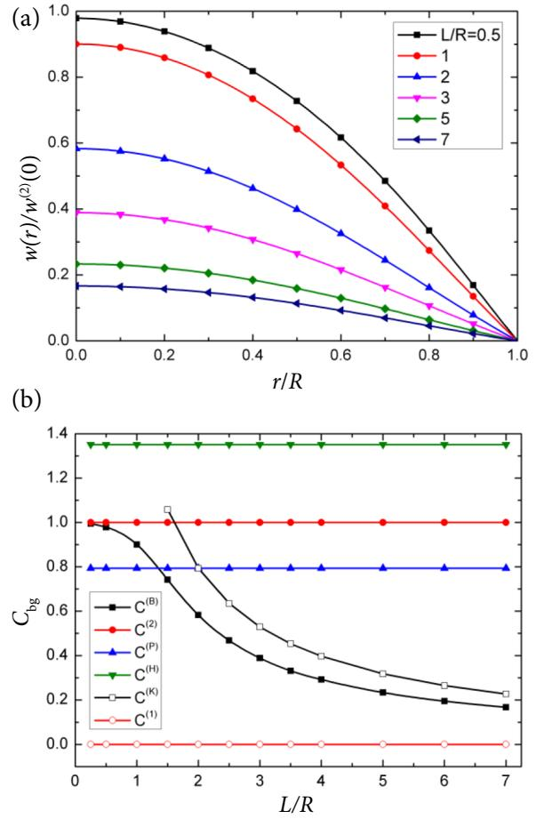
Fig. 5. Normalized bulging of the end faces for various lengths of the AE with the same radius  $R = 2$  mm (a) and dependence of bulging coefficients on the length of the AE according to various approximations (b).
