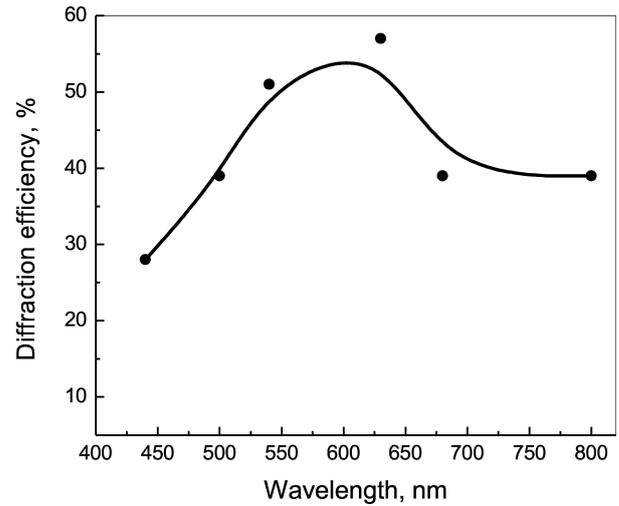
Fig. 6. Diffraction efficiency dependence on incident wavelength for a grating that is 45  $\mu\text{m}$  thick.
