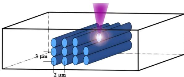
Fig. 4. Schematic layout of fabricated volume phase gratings.
