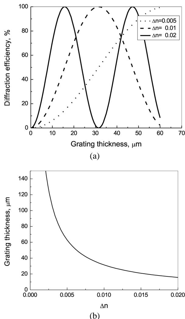
Fig. 2. (a) Diffraction efficiency dependence on grating thickness at various refractive index modulation levels; (b) dependence of minimal thickness of volume grating that produces 100% efficiency on refractive index modulation level.
