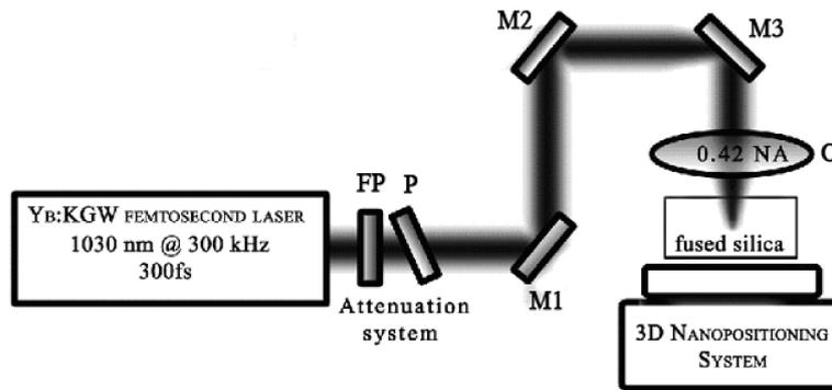
Fig. 3. Schematic of optical set-up for VPG writing. *FP* and *P* correspond to face plate and polarizer, *M1–M3* are guiding mirrors, *O* is the objective. Laser beam diameter at objective is 3.6 mm.
