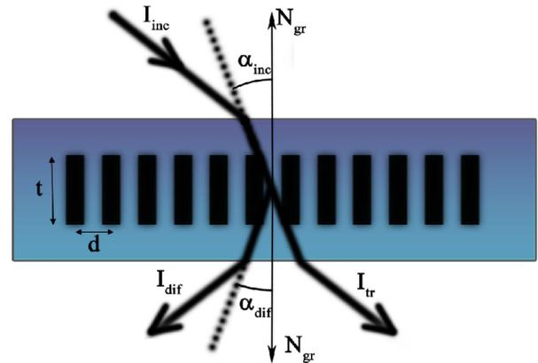
Fig. 1. Schematics of transparent volume phase grating. The equally spaced black stripes represent the region of sinusoidally modulated refractive index.
