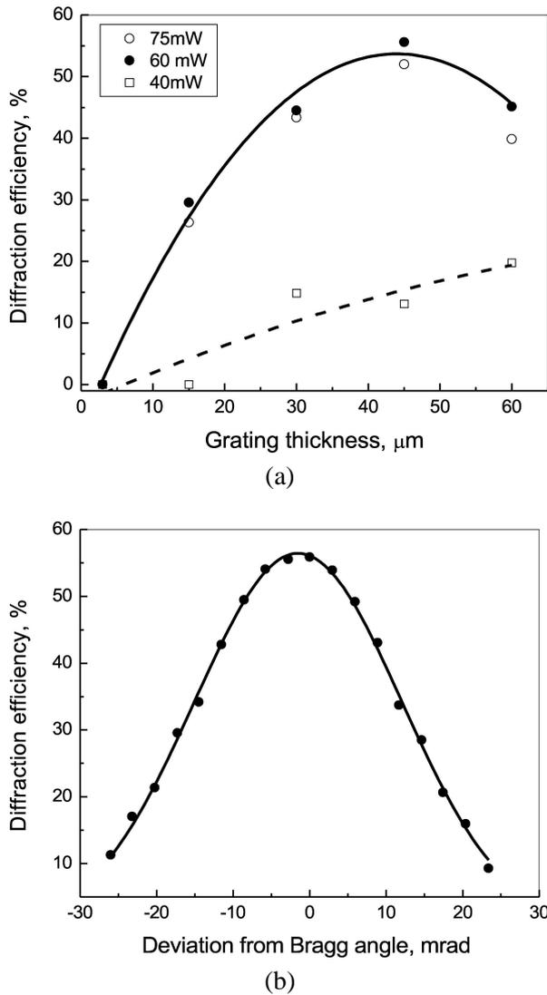
Fig. 5. Diffraction efficiency dependence (a) on the grating thickness with different writing powers and (b) on the detuning from the Bragg angle. Bragg angle was  $6.2^\circ$ . Efficiency was measured with 633 nm He-Ne laser, comparing the intensities of diffracted and incident beams.
