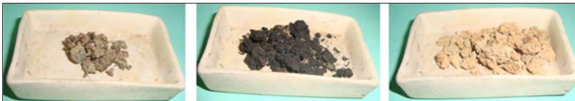
Fig. 1. The types of sludge and its residues after technical analysis: a – obsolete sludge, b – obsolete sludge after removal of volatile, c – ash obsolete sludge
