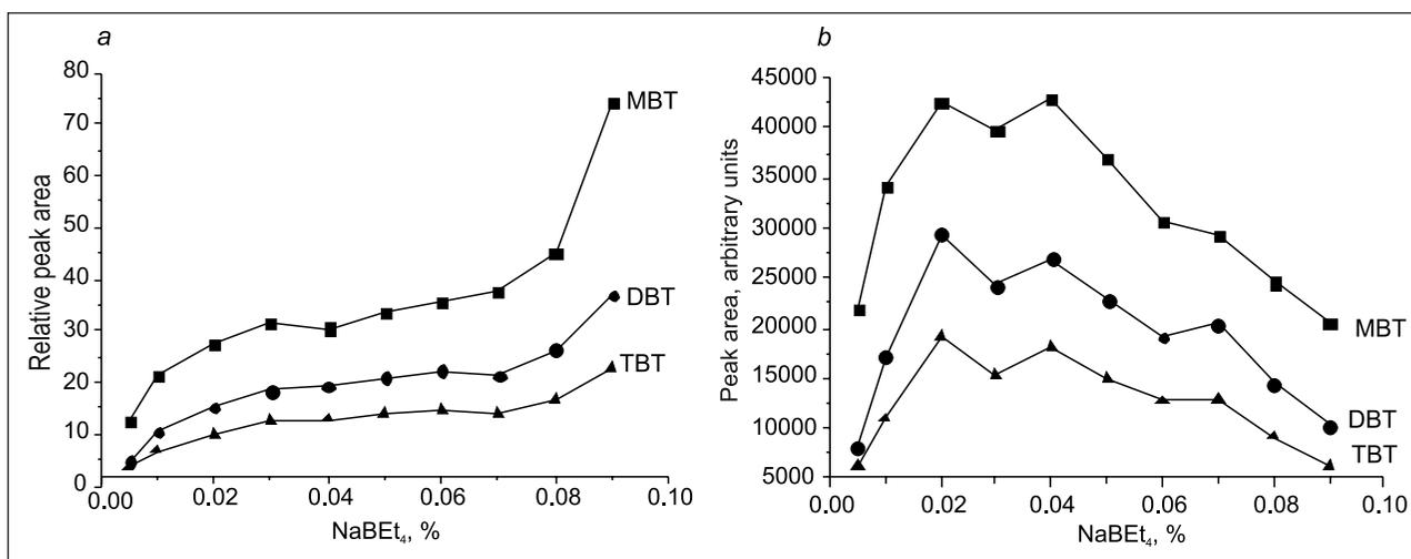
Fig. 3. Effect of the derivatization reagent concentration on the relative peak areas (a) and absolute peak areas (b) of butyltins. Sample volume 8 mL, concentration of butyltins  $10 \mu\text{g L}^{-1}$ , methanol volume  $780 \mu\text{L}$ ,  $\text{CCl}_4$  volume  $20 \mu\text{L}$ , internal standard *n*-hexadecane ( $1 \mu\text{g mL}^{-1}$  in  $\text{CCl}_4$ ), derivatization time 5 min
