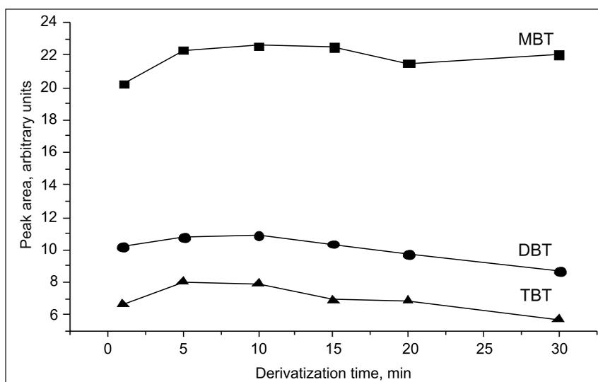
Fig. 1. Effect of the derivatization time on the derivatization efficiency
