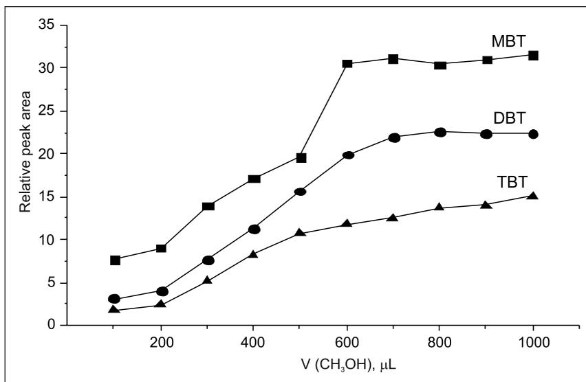
Fig. 2. Effect of the disperser solvent (methanol) volume on the DLLME efficiency. Sample volume 8 mL, concentration of butyltins  $10 \mu\text{g L}^{-1}$ ,  $\text{CCl}_4$  volume  $20 \mu\text{L}$ , internal standard *n*-hexadecane ( $1 \mu\text{g mL}^{-1}$  in  $\text{CCl}_4$ )
