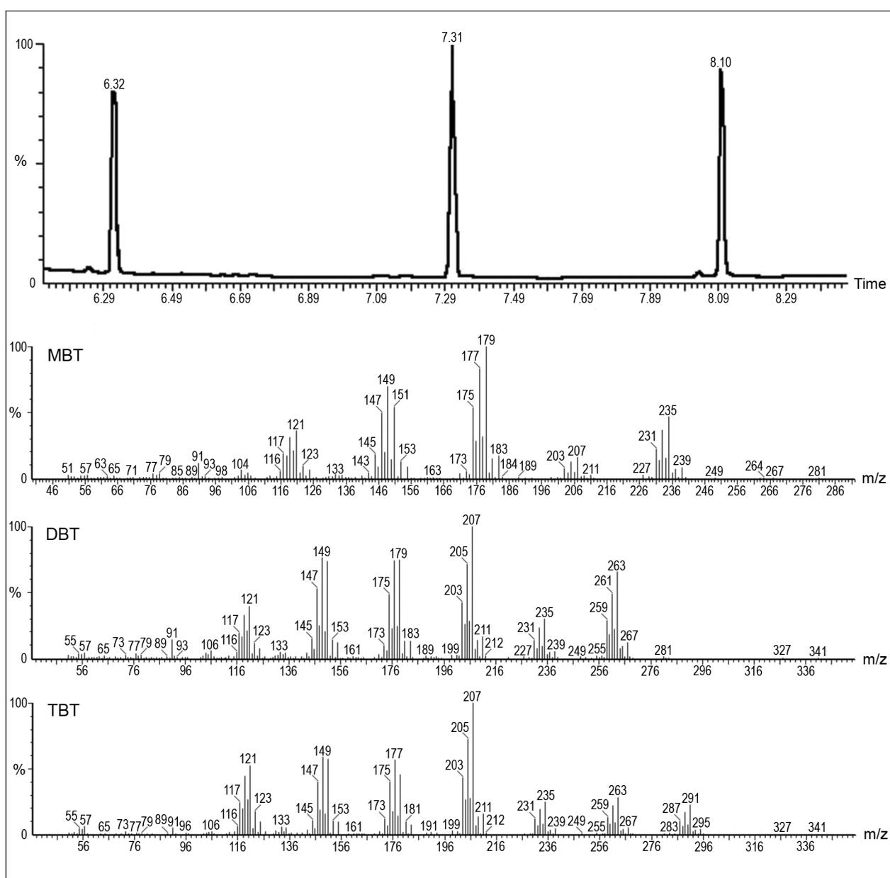
Fig. 4. Total ion GC-MS chromatogram and mass spectra of the ethylated standard mixture of MBT, DBT and TBT. For GC-MS conditions, see Experimental
