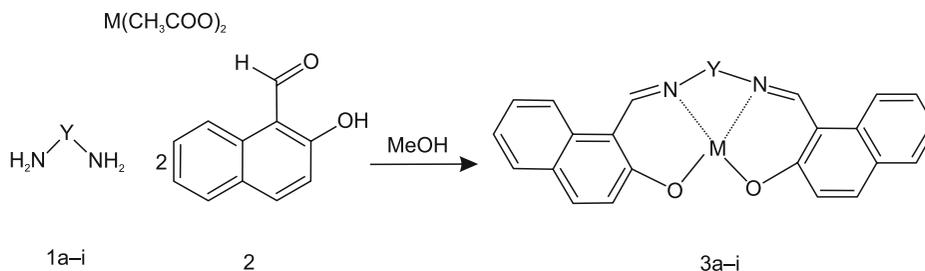
Scheme 1. Synthesis of Schiff base complexes of metal (II)
