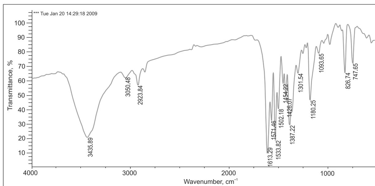
Fig. 1. The IR spectra of 1,1'-(4,4'-diphenylmethane)bis(nitrilomethylidene)-2-naphthol ligand
