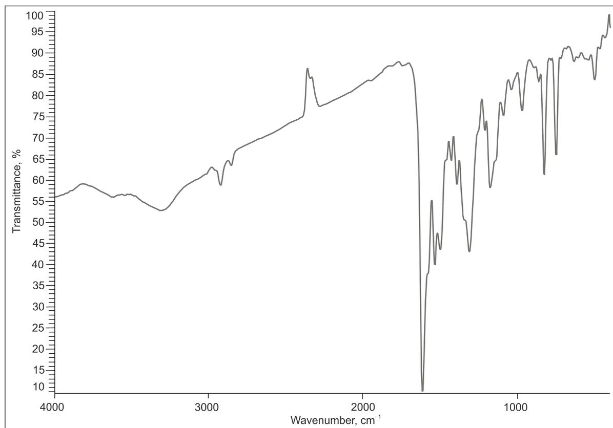
Fig. 2. The IR spectra of complex 1,1'[4,4'-diphenylmethanebis(nitrilomethylidene)]bis-2-naphtholatocobalt (II) (3h)
