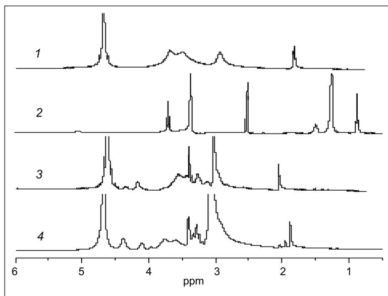
Fig. 2.  $^1\text{H}$  NMR spectra of chitosan (1), SCC (2), *O*-HTCC (DQ 28%) (3) and *N*-HTCC (DQ 68%) (4). The spectra of chitosan, *N*-HTCC and *O*-HTCC were recorded in  $\text{D}_2\text{O}$  while that of SCC in  $\text{DMSO-d}_6$ .
