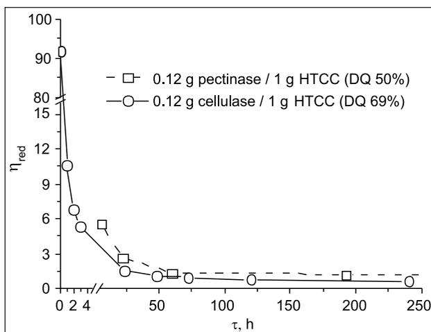
Fig. 6. Reduced viscosity of the 4% solution of *N*-HTCC versus the time of enzymatic hydrolysis at 18 °C
