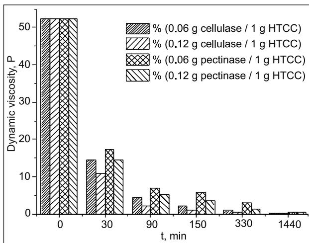
Fig. 4. Dynamic viscosity of the 4% solution of *N*-HTCC (DQ 40%) in acetate buffer versus the amount of pectinase from *Aspergillus niger* or cellulase from *Trichoderma reesi* and the time of enzymatic hydrolysis at 18 °C
