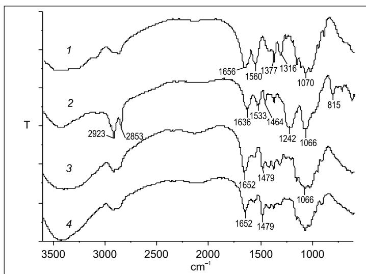
Fig. 1. FT-IR spectra of chitosan (1), SCC (2), *O*-HTCC (DQ 28%) (3) and *N*-HTCC (DQ 68%) (4)
