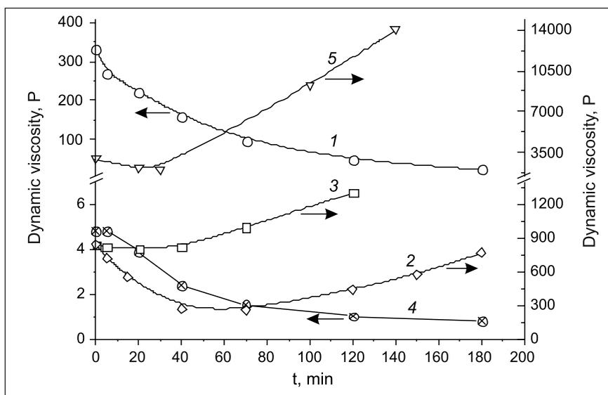
Fig. 3. UV irradiation of the 7% solution of *N*-HTCC with DQ 49% (1), 40% (2, 3), 68% (4) and 30% (5). The distance from the lamp to the quartz tube was 24 cm (1, 2, 4, 5) and 35 cm (3)
