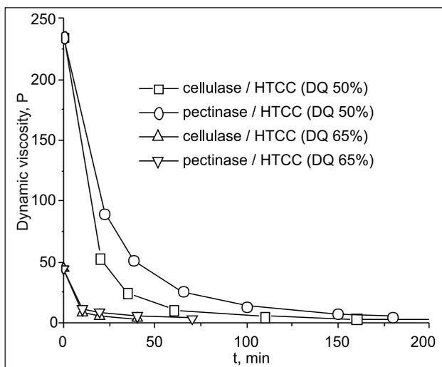
Fig. 5. Dynamic viscosity of the 7% solution of *N*-HTCC in acetate buffer versus the enzyme type and the time of enzymatic hydrolysis at 18 °C (0.12 g of enzyme to 1 g of HTCC)
