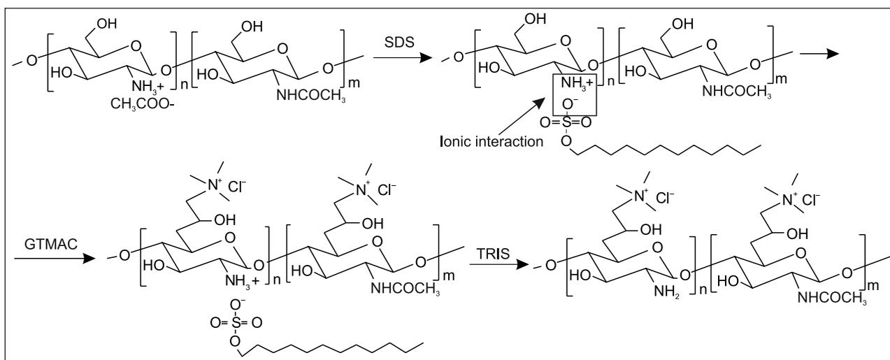
Scheme 2. *O*-Quaternization of chitosan through sodium dodecyl sulfate–chitosan complex intermediate
