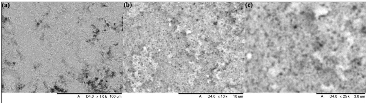
Fig. 2. SEM micrographs of the YSZ coating annealed at 800 °C temperature after 30 coating procedures on the corundum substrate
