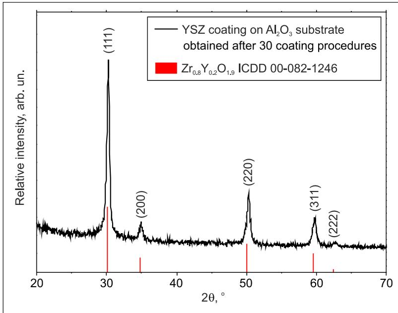
Fig. 1. Standard ICDD card of  $Zr_{0.8}Y_{0.2}O_{1.9}$  and the XRD pattern of the YSZ coating annealed at 800 °C temperature
