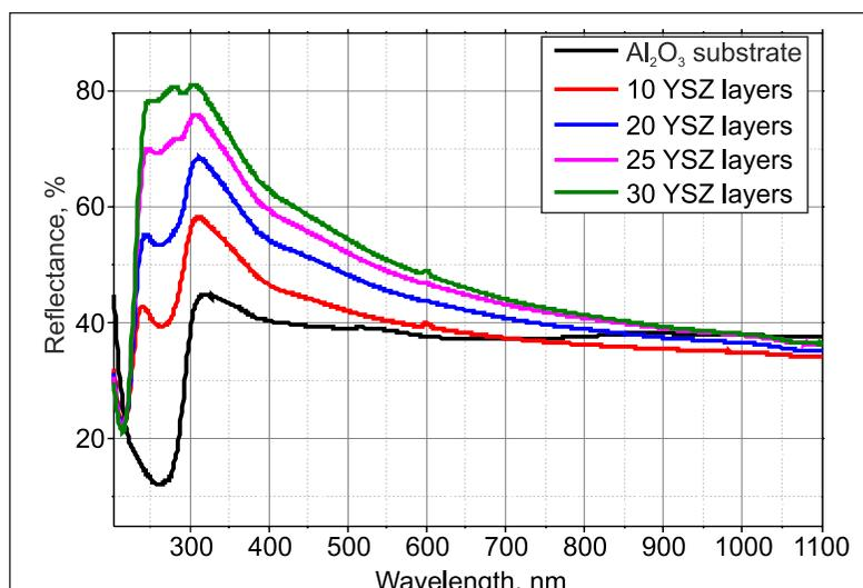
Fig. 3. UV-Vis reflectance spectra of the YSZ coatings on the corundum substrate obtained from the Y-Zr-O nitrate-propandiolate sol
