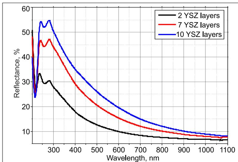
Fig. 5. UV-Vis reflectance spectra of the YSZ coatings on the silica substrate obtained from Y-Zr-O nitrate-propandiolate sol
