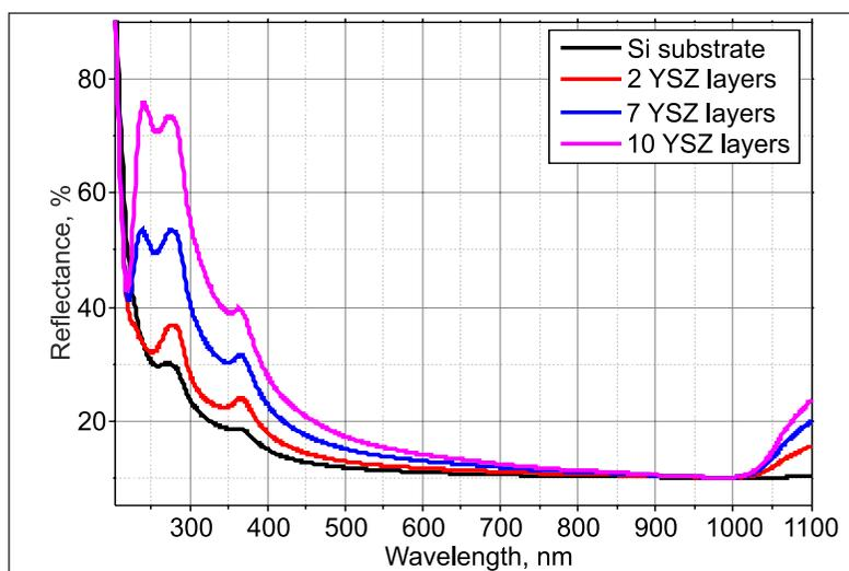
Fig. 4. UV-Vis reflectance spectra of the YSZ coatings on the silicon substrate obtained from Y-Zr-O nitrate-propandiolate sol
