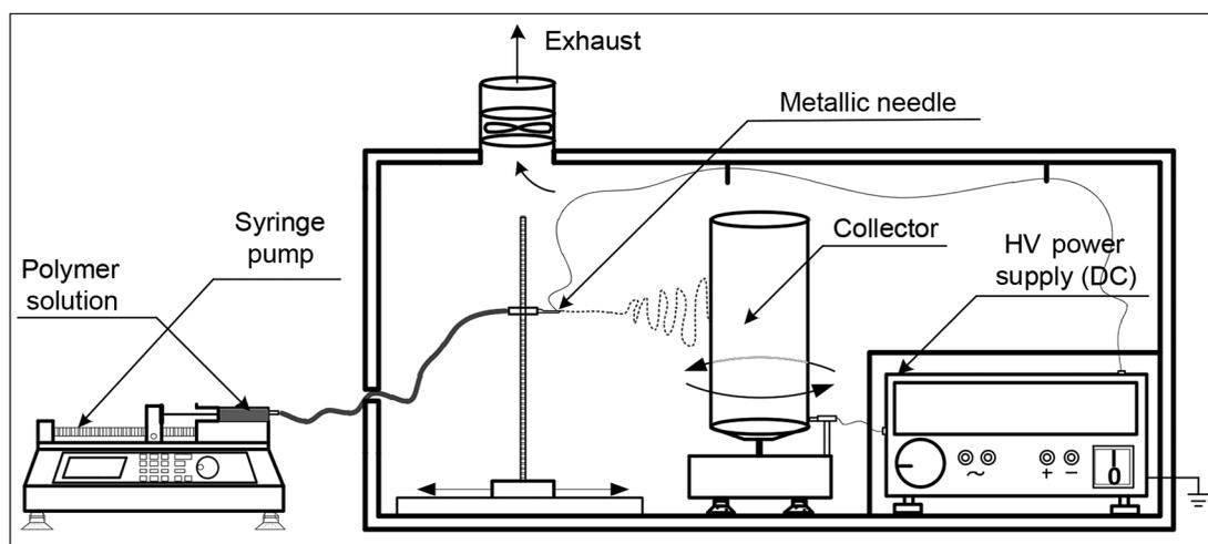
Fig. 1. Scheme of the used electrospinning system
