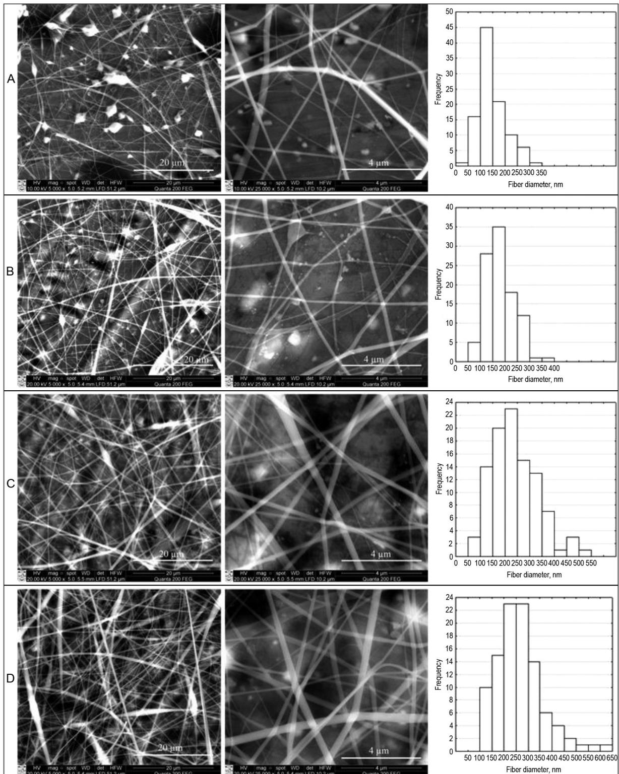
Fig. 2. SEM images of the electrospun CA nanofibers obtained from the acetone/DCM/DMF ternary solvent system and fiber diameter distribution histograms: CA concentrations – (A) 9% w/v, (B) 10% w/v, (C) 11% w/v, (D) 12% w/v
