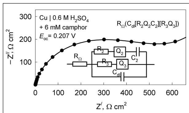
Fig. 1. Comparison of the experimental Nyquist plot (symbols) and that simulated for the given equivalent circuit (line). The EC parameters are given in the text
