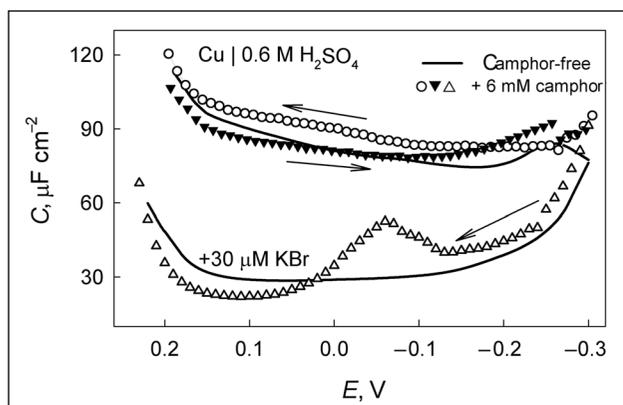
**Fig. 2.** Capacitance curves obtained for Cu(II)-free solutions containing supporting 0.6 M H<sub>2</sub>SO<sub>4</sub> electrolyte (upper part) and that with the addition of 30 μM KBr (lower part). The data obtained in the presence of 6 mM camphor are shown by symbols as indicated
