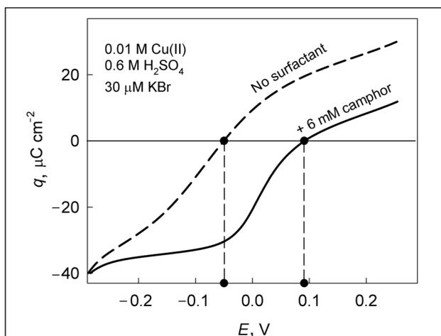
Fig. 5. Estimation of surface charge density performed by integration of capacitance curves
