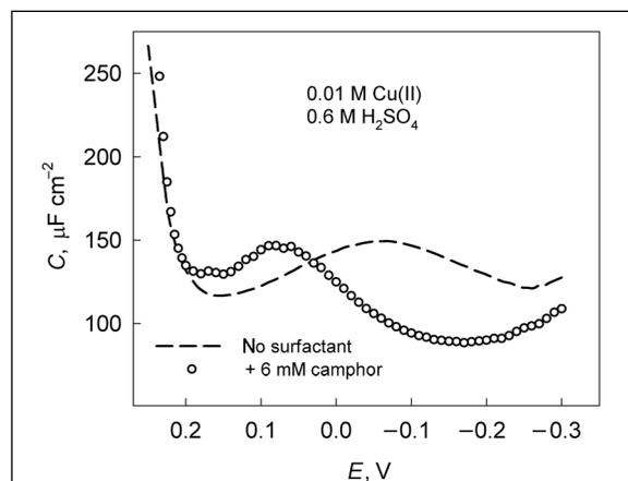
**Fig. 3.** Pseudo-capacitance curves obtained for surfactant-free (dotted line) and camphor-containing (symbols) 0.01 M Cu(II) solutions
