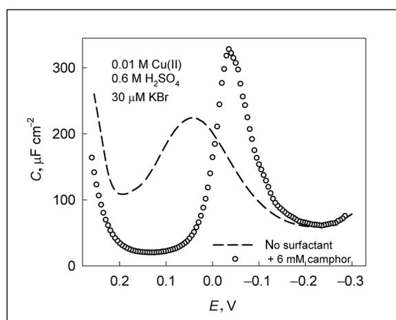
**Fig. 4.** Effect of bromide on pseudo-capacitance curves obtained for surfactant-free (dotted line) and camphor-containing (symbols) 0.01 M Cu(II) solutions
