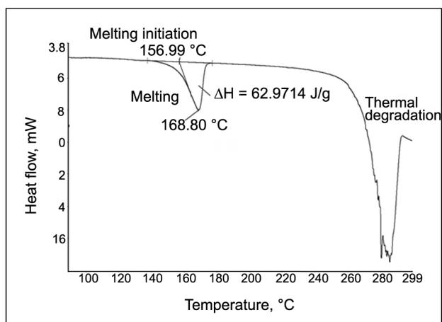
Fig. 5. The DSC thermogram of the polymer purified from *Geobacillus* sp. AY946034
