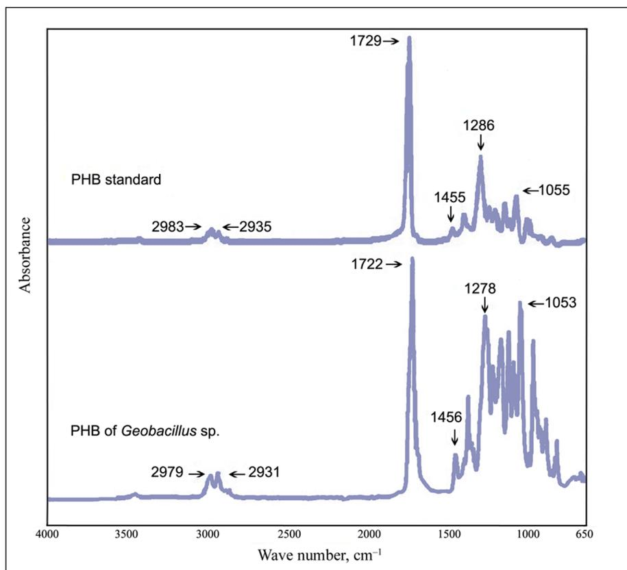
Fig. 4. FTIR spectra of PHB standard (upper) and PHB extract (bottom) from *Geobacillus* sp. AY946034 cultured with glucose as the carbon source
