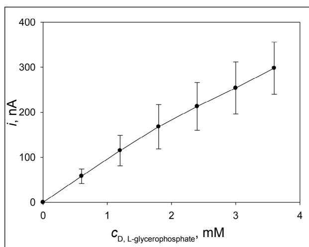
**Fig. 3b.** Dependence of the current responses of CPY<sub>bulk</sub> (sample BY3) on the concentration of D,L-glycerophosphate in de-oxygenated phosphate buffer at pH 7.3 containing 0.5 mM  $K_3[Fe(CN)_6]$ , operating potential 0.3 V
