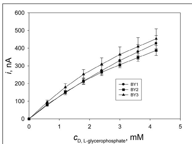
**Fig. 3a.** Dependence of current responses of CP/Y on the concentration of D,L-glycerophosphate in de-oxygenated phosphate buffer at pH 7.3 containing 0.5 mM  $K_3[Fe(CN)_6]$ , operating potential 0.3 V
