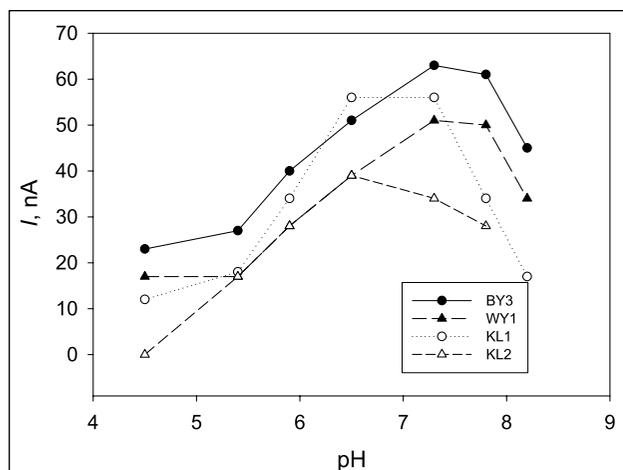
**Fig. 2.** Dependence of the current responses of CP/Y on solution pH in de-oxygenated phosphate buffer containing 0.6 mM D,L-glycerophosphate and 0.5 mM  $K_3[Fe(CN)_6]$ , operating potential 0.3 V
