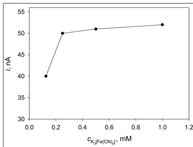
Fig. 1. Dependence of the current responses of CP/Y (sample BY1) on the concentration of K<sub>3</sub>[Fe(CN)<sub>6</sub>] in de-oxygenated phosphate buffer at pH 7.3 containing 0.6 mM D,L-glycerophosphate, operating potential 0.3 V
