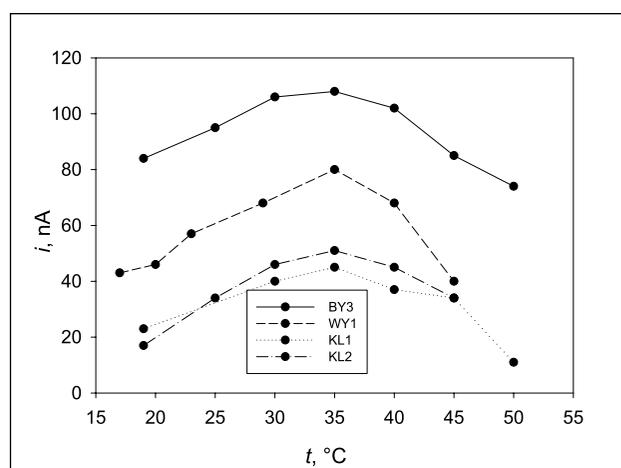
**Fig. 4.** Dependence of the current responses of CP/Y on the temperature in de-oxygenated phosphate buffer at pH 7.3 containing 0.6 mM D,L-glycerophosphate and 0.5 mM  $K_3[Fe(CN)_6]$ , operating potential 0.3 V
