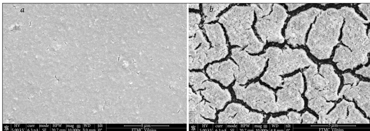
**Fig. 4.** FESEM views of CdS, formed on the glassy carbon from the ethylene glycol (a) and 2-propanol (b) solutions by spin-coating. The CdS nanocrystals were prepared from the reaction mixture containing  $0.1 \text{ mol l}^{-1} \text{ Cd}(\text{NO}_3)_2$ ,  $0.2 \text{ mol l}^{-1} \text{ CH}_4\text{N}_2\text{S}$ ,  $0.005 \text{ mol l}^{-1} \text{ EDTA}$ ; pH 8.5. Parameters of microwave synthesis:  $t = 100 \text{ }^\circ\text{C}$ ;  $P = 100 \text{ W}$ ,  $\tau = 10 \text{ min}$
