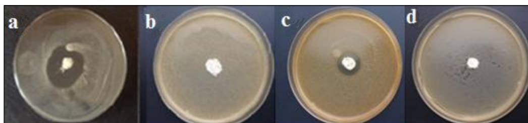
Fig. 9. Pictures of Petri dishes with MgO nanoparticles in Saccharomyces cerevisiae culture (a), Escherichia coli culture (b) and bare MgO in Saccharomyces cerevisiae culture (c), Escherichia coli culture (d)
