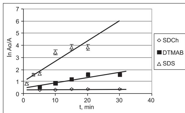
Fig. 3. The lipase-catalysed hydrolytic reaction affected by ionic detergents. Inactivation rate constants of the reaction upon p-NPB solution in propan-2-ol,  $k_{\text{inact}}$   $\text{min}^{-1}$ : SDS – 0.290; DTMAB – 0.070; SDCh – 0.006
