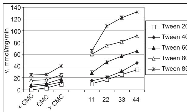
**Fig. 2.** The effect of Tween physical state in the reaction mixture on the lipase hydrolytic activity. The activity was determined by the standard titrimetric method at the following final Tween concentrations: two-fold below CMC, close to CMC, five-fold above CMC and far exceeding CMC (11–44 mM)
