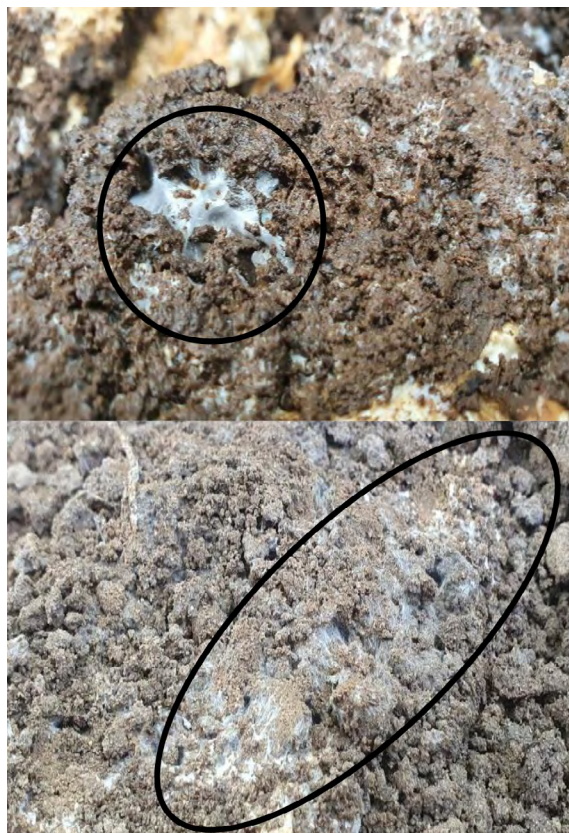
Fig. 9. Growth of mycelium over the biomaterial kept for biodegradation
