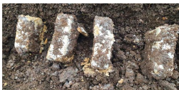
Fig. 8. Biomaterial observed after 30 days of biodegradation
