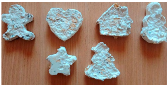
Fig. 10. Shaped biomaterials made from sawdust and buckwheat substrate combination
