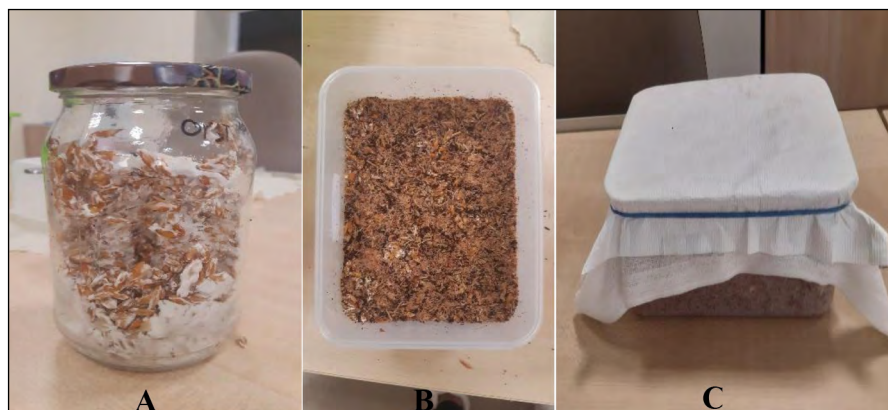
Fig. 1. Sample preparation to produce a biomaterial block. A – stock culture, B – sample mixed with substrate and fungal mycelium placed in the container, C – sample covered with muslin cloth and a polyethylene sheet
