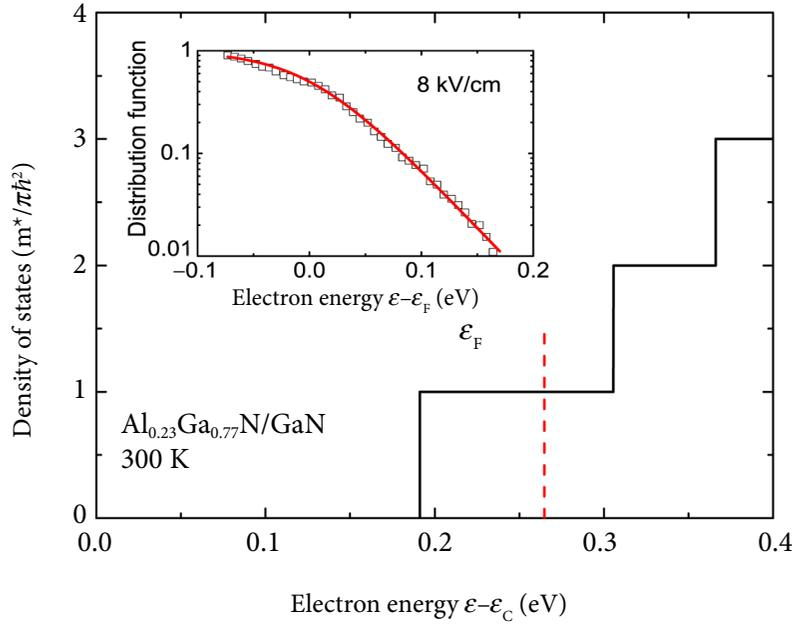
Fig. 1. Density of states for subbands in  $\text{Al}_{0.23}\text{Ga}_{0.77}\text{N}/\text{GaN}$  at temperature of 300 K. Red online dashed line stands for the Fermi energy. Inset illustrates the electron distribution function in the lowest subband at electric field of 8 kV/cm: the Fermi–Dirac approximation at hot-electron temperature of 440 K (red online curve) fits the results of Monte Carlo simulation (squares).
