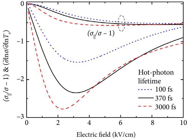
Fig. 2. Dependence of the steady-state electric sensitivity  $\partial \ln \sigma / \partial \ln T_e$  and the measure of non-ohmic behaviour  $\sigma_{\parallel} / \sigma - 1$  on the electric field obtained from the analysis of Monte Carlo results for the model shown in Fig. 1 for three values of hot-phonon lifetime: 100 fs (blue online dotted curve), 370 fs (solid black curve), and 3000 fs (red online dashed curve).
