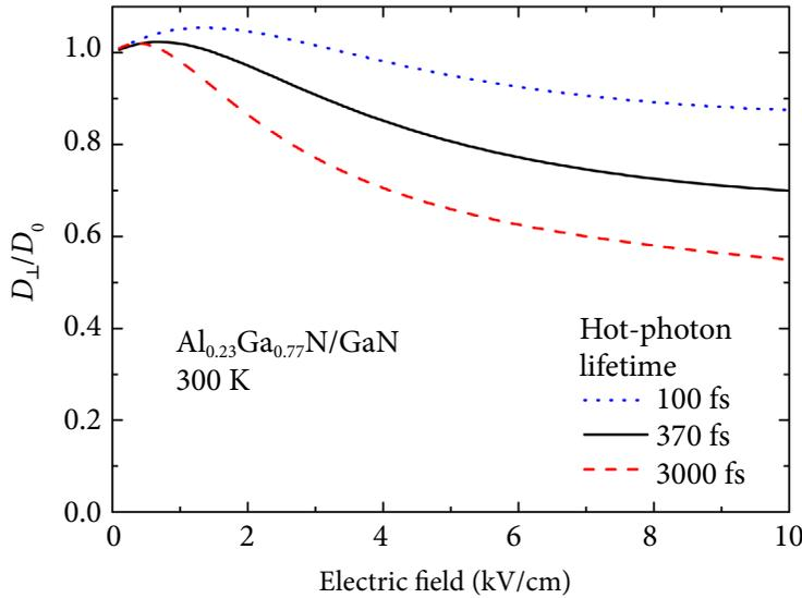
Fig. 3. The coefficient of steady-state transverse diffusion for the  $\text{Al}_{0.23}\text{Ga}_{0.77}\text{N}/\text{GaN}$  model at 300 K based on the Monte Carlo simulation for three assumed values of hot-phonon lifetime: 100 fs (blue online dotted curve), 370 fs (solid black curve), and 3000 fs (red online dashed curve).
