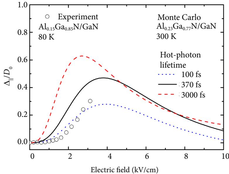
Fig. 4. The coefficient of additional correlation in the electron temperature approximation for the  $\text{Al}_{0.23}\text{Ga}_{0.77}\text{N}/\text{GaN}$  model at 300 K based on the Monte Carlo simulation for three assumed values of hot-phonon lifetime: 100 fs (blue online dotted curve), 370 fs (solid black curve), and 3000 fs (red online dashed curve). Open circles stand for experimental data at 80 K for the  $\text{Al}_{0.15}\text{Ga}_{0.85}\text{N}/\text{GaN}$  structure [20].
